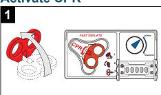
Lift the red handle on the control panel at foot end of the mattress.
