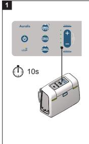
When the pump is connected to a power source it runs a self check: Beep – 10 seconds – 2 beeps – ready to use.
