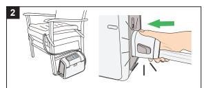
Place pump on floor, cable under chair, tubeset placed alongside chair.
