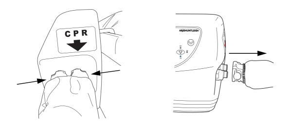
Located on the right hand side of the pump is a CPR device marked with an arrow. In the event of cardiac arrest, press the two quick release catches on the tubeset/pump connector, and simultaneously pull the hose away from the pump.
