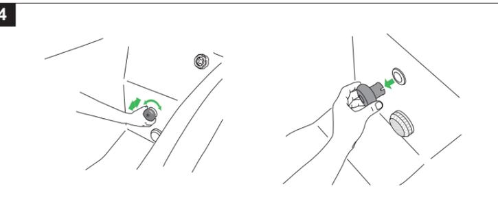
Adjust the water jet direction by turning the outlet. Pull out the adjustable nozzle to get the jet to cover a wider area.
