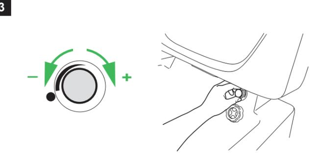
Adjust the water flow with the intensity level knob. Start with low intensity, turn clockwise to increase.
