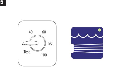
Start with a low intensity level. Turn clockwise to increase. The LED shows a steady green light and a buzzing sound is heard when any active level is selected.
