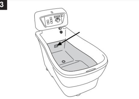
Make sure the water level is above the top of the Hydrosound system transducer plate.
