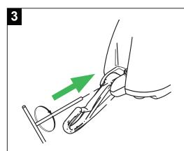
Insert the special tool into the opening. Turn it clockwise to lower the patient. The tool rotation turns the motor directly, so that for each tool turn, the patient will lower slightly.
