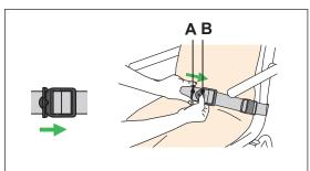
Lock fastening clip. Lock the fastening clips by inserting the smaller fastening clip (A) into the larger fastening clip (B).
