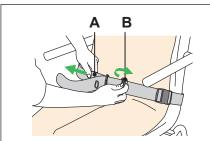
Loosen the safety belt. Pull the inner strap (A) at the side while lifting the larger fastening clip (B).
