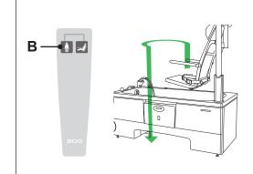
Push and hold the Lift out button **(B)**. The sequence will be performed in the reverse order.
