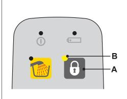
Push and hold the patient lock out button (A) for 3 seconds to disable all panel and remote buttons. Patient lock-out is indicated by a yellow LED (B).
