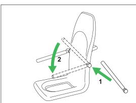
Hold the armrest with the handle pointing up wards. Guide the armrest slots onto the transfer chair (1).
