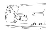
The massage effect is obtained by injecting air through air jets into the bath water. The recommended maximum treatment with the Air spa system is 15 minutes.
