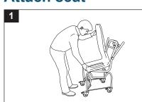
With both hands start pushing the front end of the seat against the front frame.
