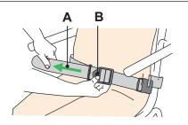
Tighten the safety belt. Pull the outer strap (A) at the side while holding the larger fastening clip (B).
