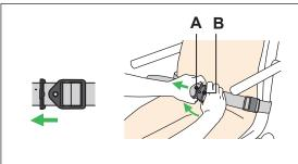
Unlock fastening clip. Pull the fastening clips (A) and (B) apart by twisting the smaller fastening clip (A) slightly upwards.
