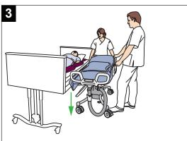
Position shower trolley next to the bed's transfer side. Fold down the shower trolley mattress on transfer side.
