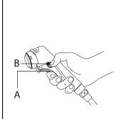
Shower handle is grey or white. Disinfection handle is red or yellow. Turn on flow control. Hold the trigger in for constant water flow (A). On shower handle, press lock button for continuous flow (B).
