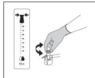
Shows mix ratio between disinfectant and water. To adjust, turn the suction part on the bottle cap. Make sure the mix is correct when starting disinfection. (See IFU.)
