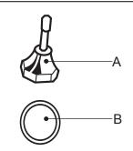
If a flush sink is connected, flush it by moving the flushing valve (A) forwards or backwards, or by pushing the flush button (B).
