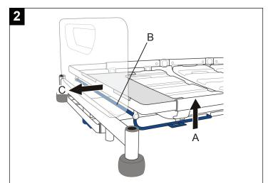
Lift the blue extension catch bar (A) and hold the middle of the crossbar (B), then pull the mattress platform to position (C).
