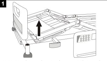
Hold side of the calf section frame and lift the calf section upwards.
