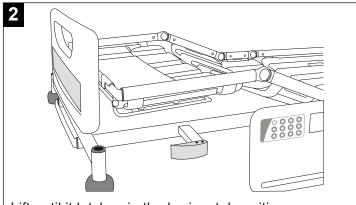
Lift until it latches in the horizontal position.
