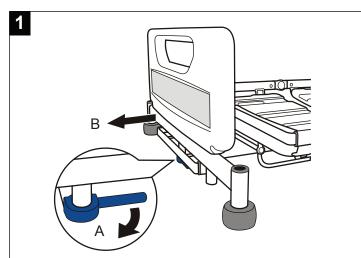
Pull the blue extension locking handle (A). Pull out the bed frame (B) to required position and release handle.
