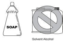
**i** Do not use petroleum based solvents or alcohol.
