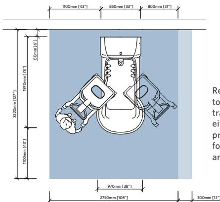
Required working area to facilitate bathing and transfer activities from either side of the tub while providing adequate access for the resident, equipment and assisting carer.
