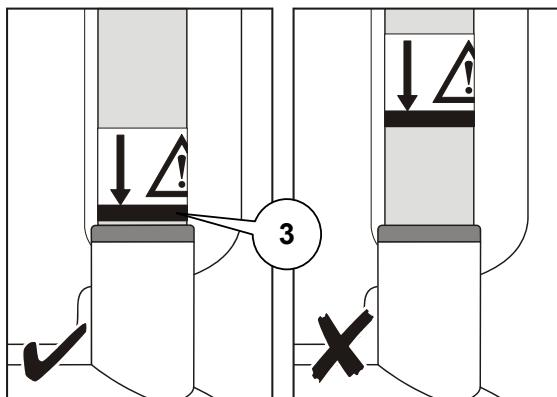
When the lifting pole is correctly installed, the indicator line (3) will be level with the top of the socket.
