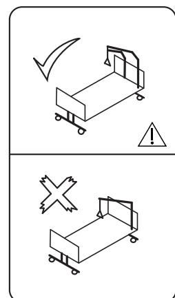
*To reduce the risk of patient entrapment, the head end panel must remain fitted at all times while the lifting poles are installed on the bed.*
