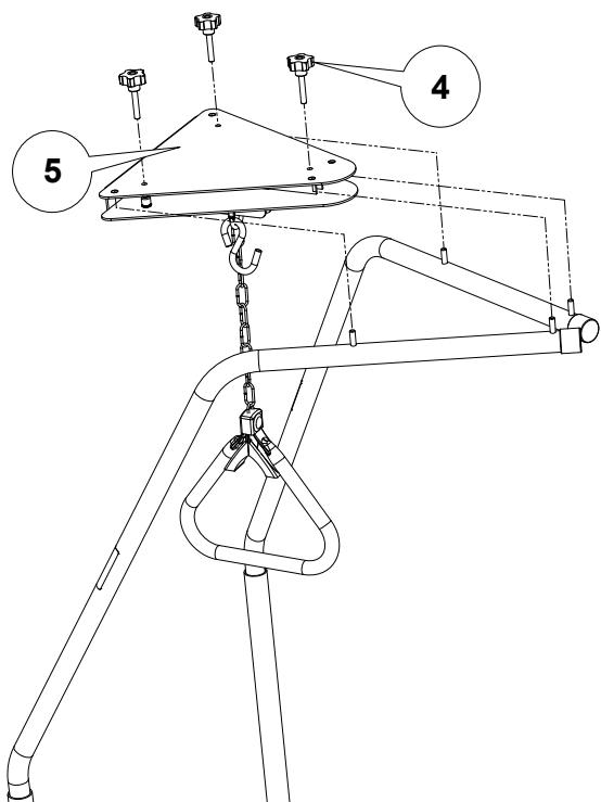
To adjust the height of the handle above the bed: press desired chain loop onto the "s" hook provided.
