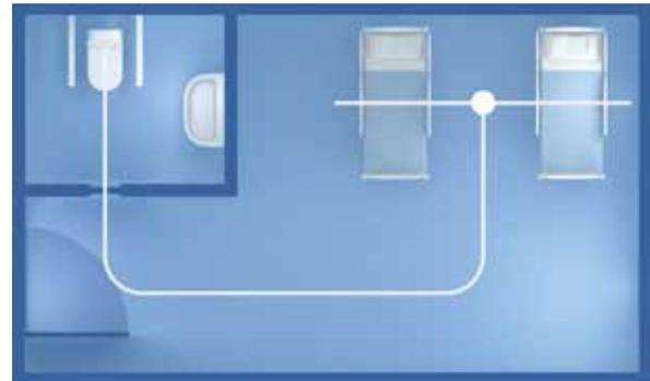
Two fixed tracks over the beds connect to a turntable and curved track section to provide access for toileting.
