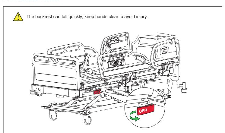
Pull the red CPR handle located on either side of the bed to quickly lower the backrest.
