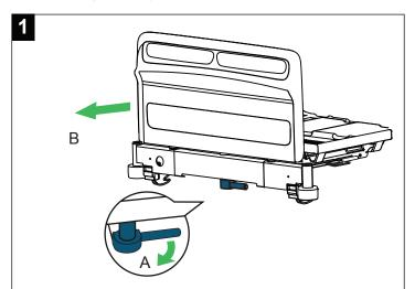
Pull the blue extension locking handle (A). Pull out the bed frame (B) to required position and release the handle.
