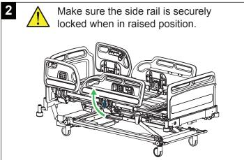
To raise side rail, hold side rail handle and pull side rail up and away from the bed until it locks in the raised position.
