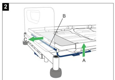
Lift the blue extension catch bar (A) and hold the middle of the crossbar (B), then pull the mattress platform to position (C).
