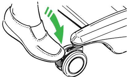
For storage and on incline only. Do not apply brakes when lifting a patient in any other way.
